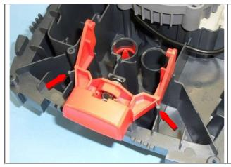
Put the locking lever together with the spring into place. See the picture on the side.
