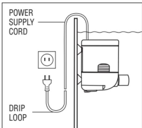
The “drip loop” is that part of the cord below the level of the receptacle, to prevent water travelling along the cord and coming in contact with the receptacle.
