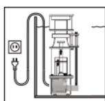
For your own safety we recommend that you make a drip loop with the power cord. This drip loop prevents any water running along the cord from reaching the electrical socket.
